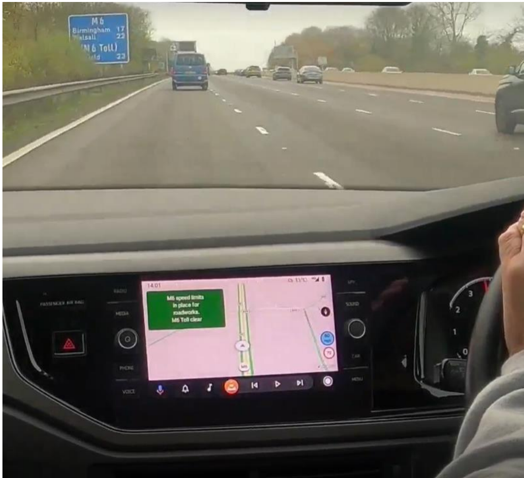
Figure 25 - Example of an in-vehicle VMS message displayed via an Android Auto connection
